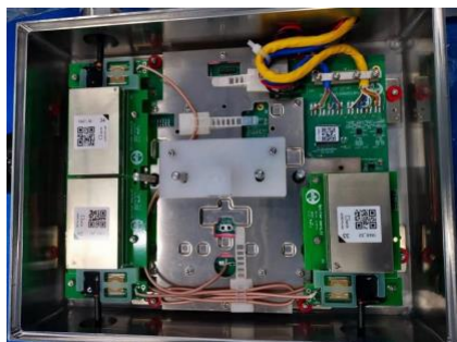
LPMTs: 3 PMTs connected to one underwater box
