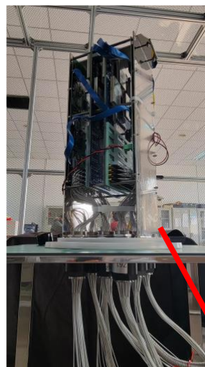
SPMTs: 128 PMTs connected to one underwater box
