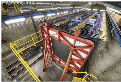
Near Detector 4m x 4m x 15.6 m underground
