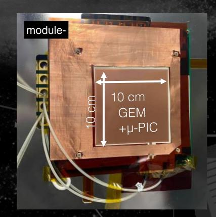
GEM + μ-PIC 10 × 10 cm<sup>2</sup> detection area read by 256 strips Track reconstruction
