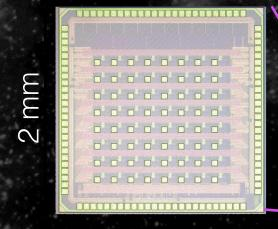
readout ASIC (155 um)<sup>2</sup> pixel pad connecting to electrodes by bump bonding
