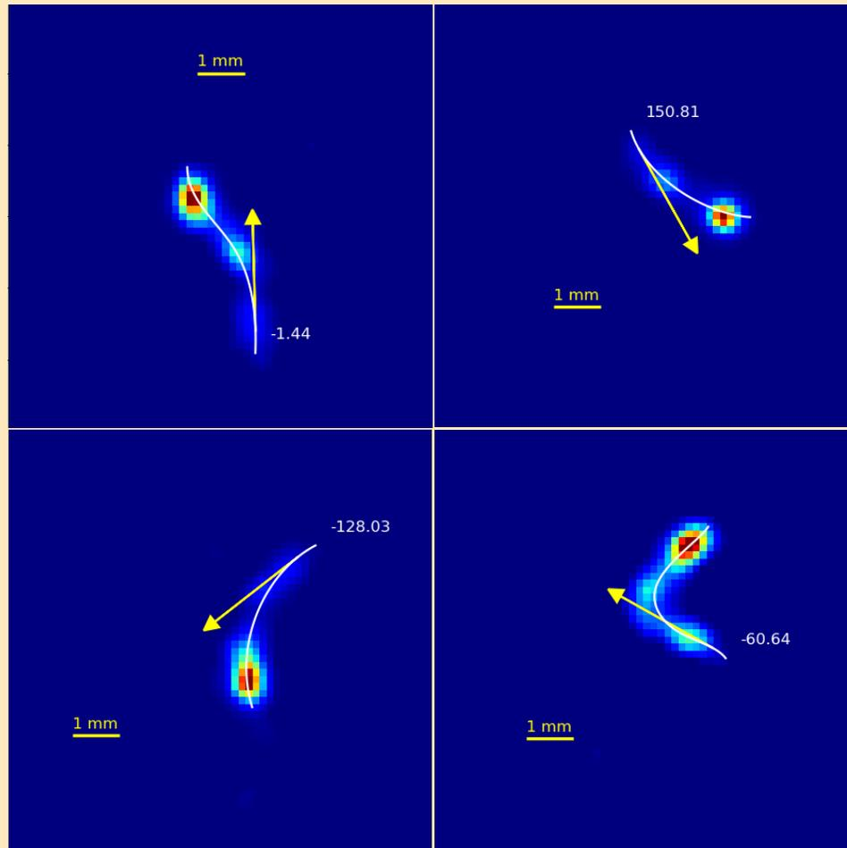
Low diffusion, high spatial resolution enables detailed reconstruction of particle's trajectory:
