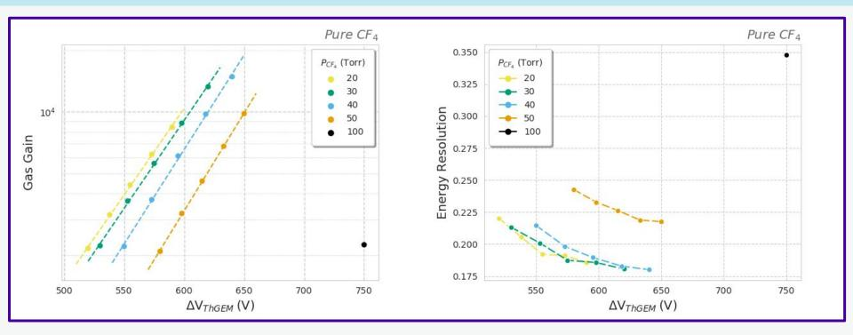
Gain curves could not be obtained for 5 and 10 Torr, only 1 data point could be obtained for 100 Torr due to narrow range of operating voltages Energy resolution found to be similar for 20, 30, and 40 Torr but increases significantly at 50 and 100 Torr
