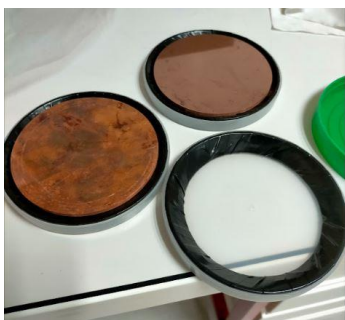
Metallographic Polishing (MP) from IJCLab courtesy of D. Longuevergne & O. Hryhorenko ( S_a \sim 20 nm, Ave S_z \sim 2.5 \mu m)
