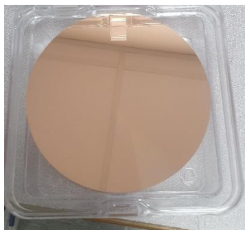
Diamond Turned (DT) from RAL ( S_a \sim 2-3 nm, S_q \sim 5-6 nm)
