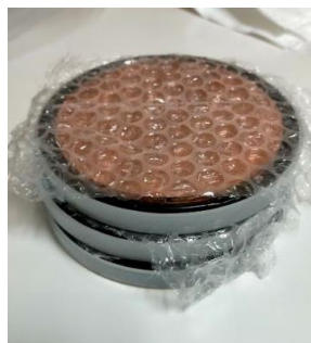
Metallographic Polishing (MP) from IJCLab courtesy of D. Longuevergne & O. Hryhorenko ( S_a \sim 20 nm, Ave S_z \sim 2.5 \mu m)
