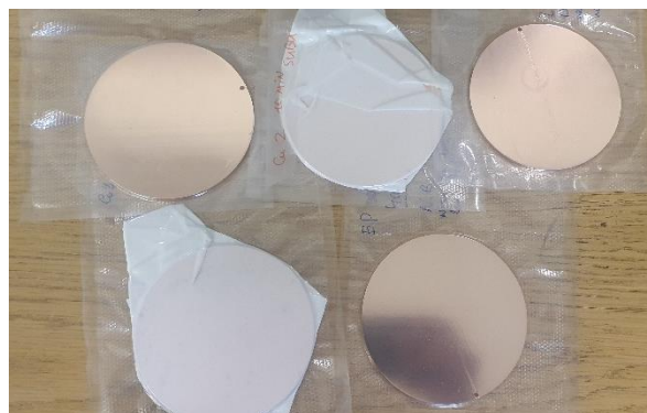
EP, SUBU, EP + SUBU from INFN courtesy of E. Chyhyrynets and C. Pira
