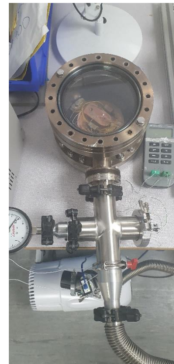
Samples are indium brazed to sample holder under vacuum at \sim 160 ^{\circ} C
