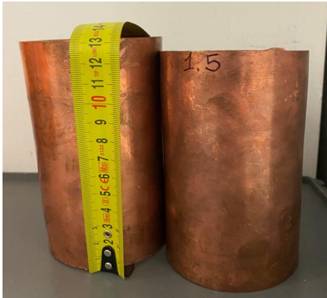
1.3 GHz cavity «tubes» For deposition and Laser Annealing
