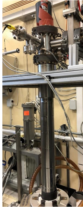
Inconel chamber replaced by a Nb chamber
