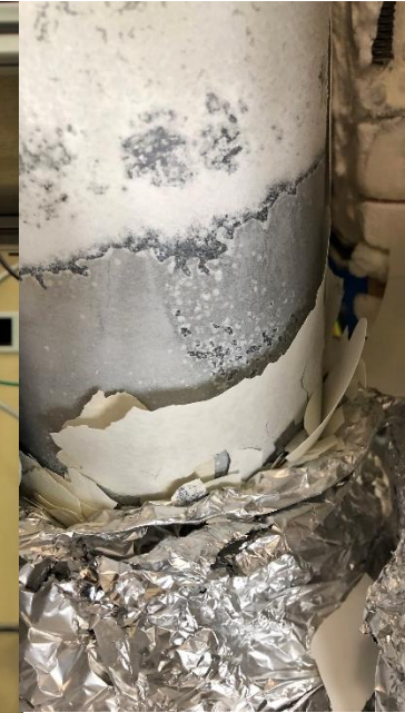
After the first test (30 min @ 1000 °C) a very thick film of Nb 2 O 5 growth on the external surface
