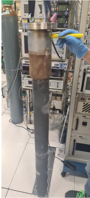
Inconel chamber replaced by a Nb chamber
