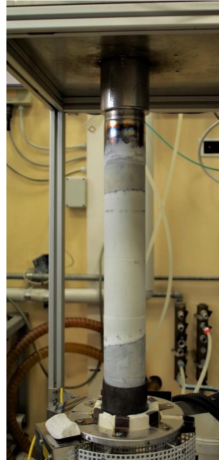
After the first test (30 min @ 1000 °C) a very thick film of Nb 2 O 5 growth on the external surface
