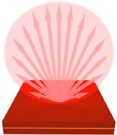
LED slab with Lambertian distribution of emission
