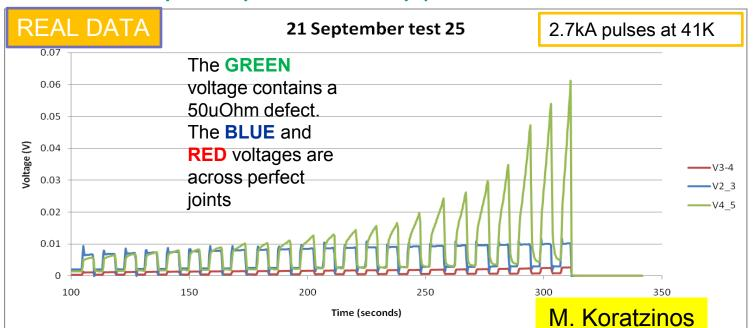
RB: a typical bad joint has excess resistance of 2% - if we warm it up, its resistance grows by ~200 times – easy to detect!
