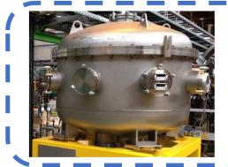
A reaction chamber to place the detectors, capable of achieving high vacuum and (ideally) previously tested.
