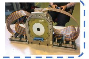
The pentagon is a particle + gamma detection system developed by the IEM experimental nuclear physics group.
