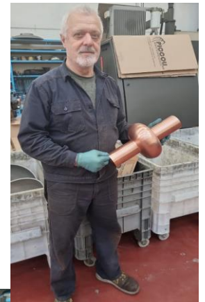
1.3 GHz seamless copper production by spinning
