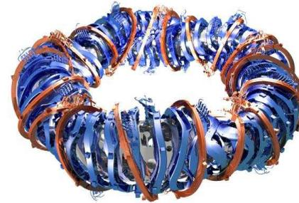
W7-X is the only stellarator in operation in EU. It is constituted by 60 superconducting NON-planar coils, 36 of which have been manufactured by ASG.
