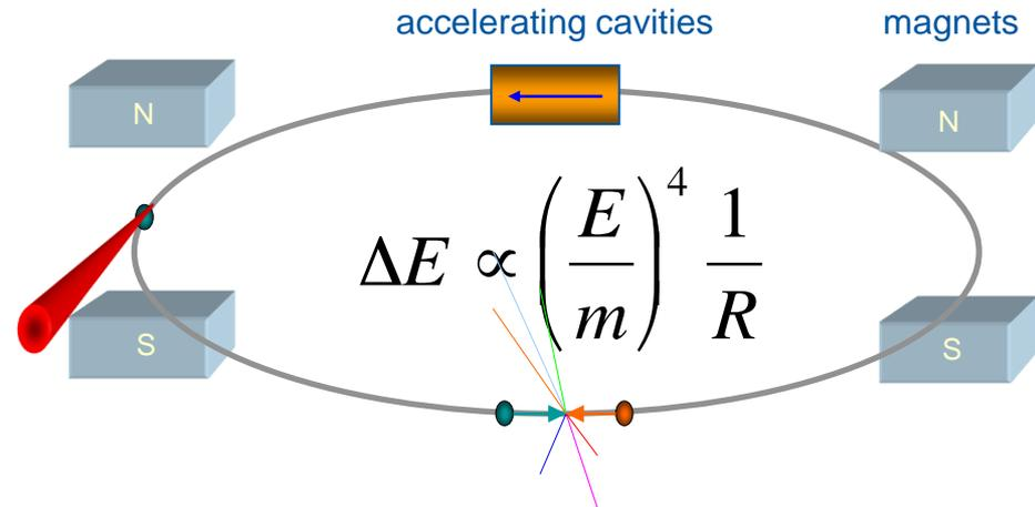
Electron-positron linear colliders **avoid synchrotron radiation**, but are **single pass**
