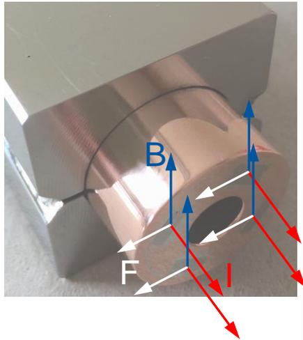
May this be the reason why soldered and twisted high field and high current cables are also subject to degradation ?
