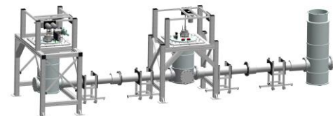
QMICS Cryolink @ 35 mK for SC cable Courtesy of Oxford Instruments and WMI
