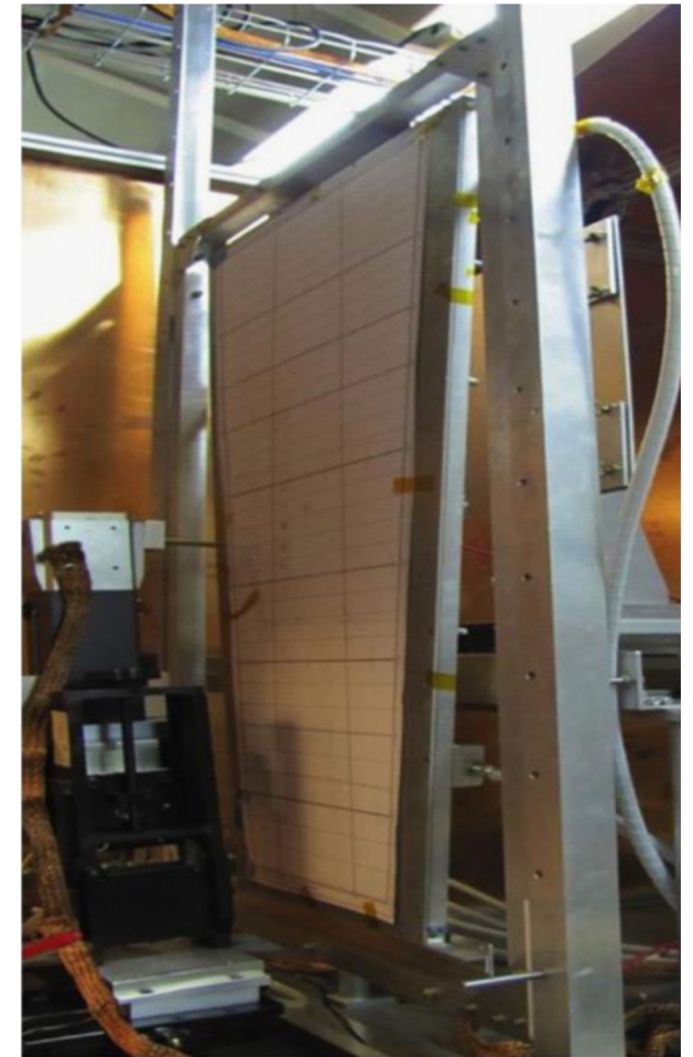
Fig. 34. A large GEM prototype for the CMS forward muon upgrade. The detector is about one meter high.
