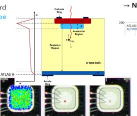
Typical Single Event Burnout mark is shown in the right plot (2019 DESY test-beam with 5 GeV e). The reconstructed track in the SEB event pointed to the location of the burn mark (middle and right plot). All the reconstructed tracks distribution across the detector before SEB is shown in the left plot.
