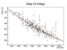
Example of delay distribution of different PMT channels as a function of applied HV power supply as resulting from the laser calibration
