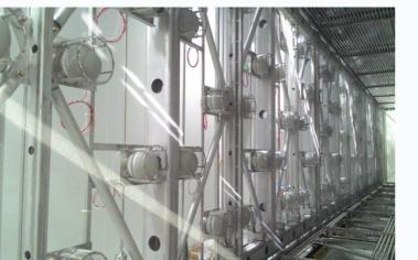
A fast-laser based calibration system has been developed for gain/time calibration, equalization and monitoring of each PMT channel. Laser pulses ( $\lambda$ =405m, FWHM 60 ps) are sent to each PMT (360) via a light distribution system.
