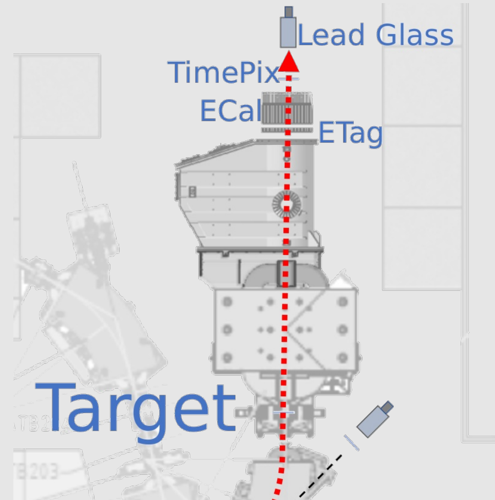
Fig. 3. PADME setup used for X-17
