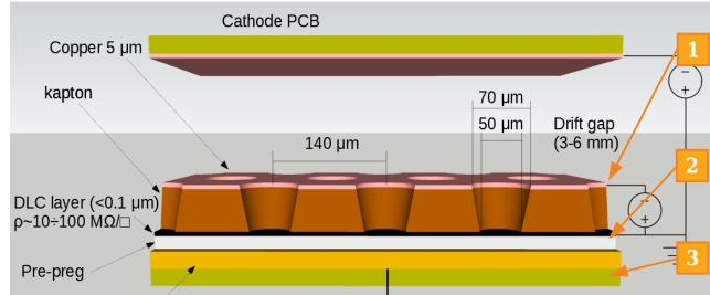
**A WELL** patterned kapton foil acting as **amplification stage**
