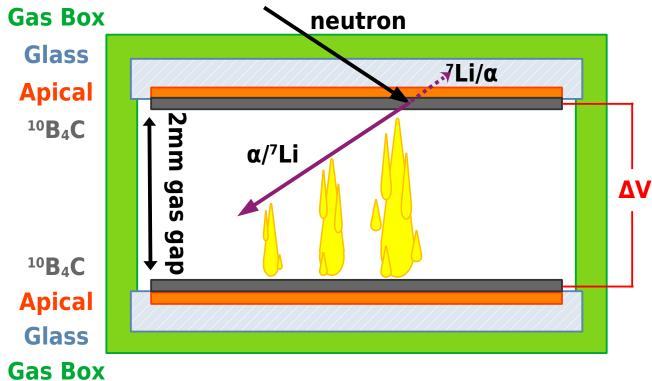
Since the <sup>10</sup>**B**<sub>4</sub>**C** surface resistivity is **O(1 M\Omega/\Box)**, it is possible to **switch** one (or both) of the DLC electrodes. The <sup>10</sup>B<sub>4</sub>C will act as a converter surface facing the gas gap, ensuring also the high voltage for detector operation.
