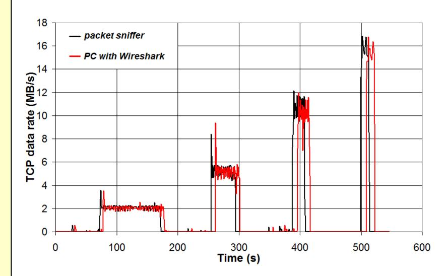
A file (Arduino IDE, file size 197 MB) has been downloaded using the Linux command "wget".
