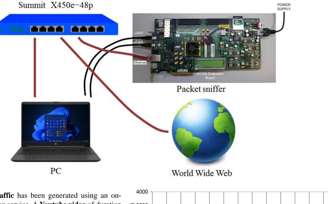
UDP Ethernet traffic has been generated using an online video streaming service. A Youtube video of duration of about 2 minutes was viewed on the PC using **different** video resolutions (1080p, 720p and 480p) and the corresponding UDP traffic monitored with the firewall hardware and Wireshark.
