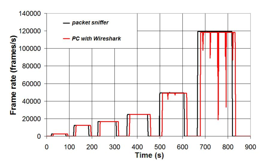
The **performance** of the proposed **firewall** have been compared with Wireshark, a popular packet sniffer software.
