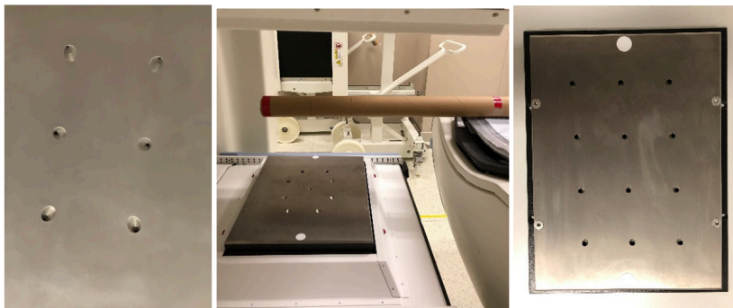
Figure. 1. 6-PH collimator (left), 9-PH collimator (middle) and 12-PH collimator (right) for small animal imaging, brain imaging and cardiac imaging in this study.
