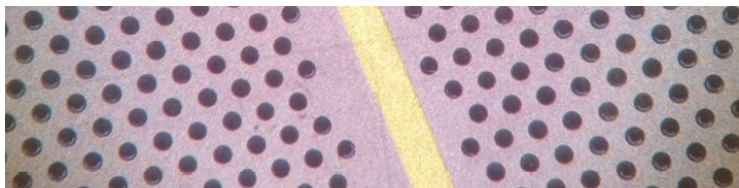
Separation between GEM foil sectors on ME0 detector seen at microscope
