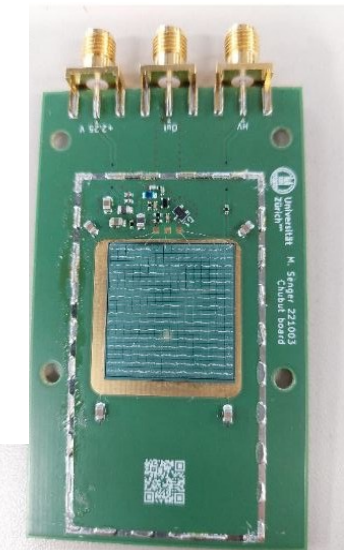
A 16x16 bonded to the UCSC-UZH board
