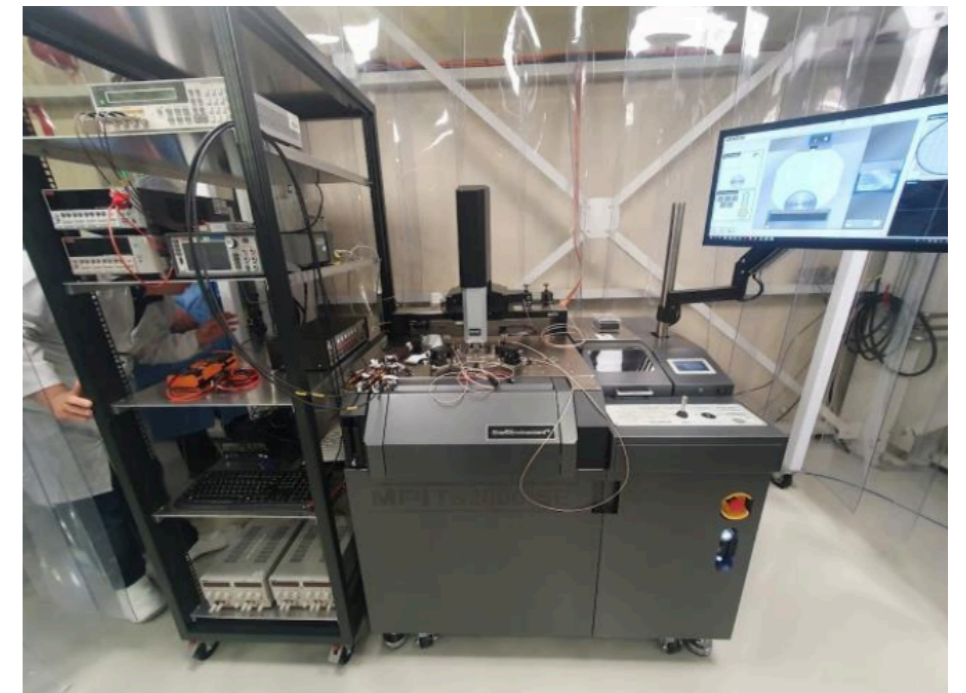
Automatic test system at CERN with dedicated probe-card and DAQ software
