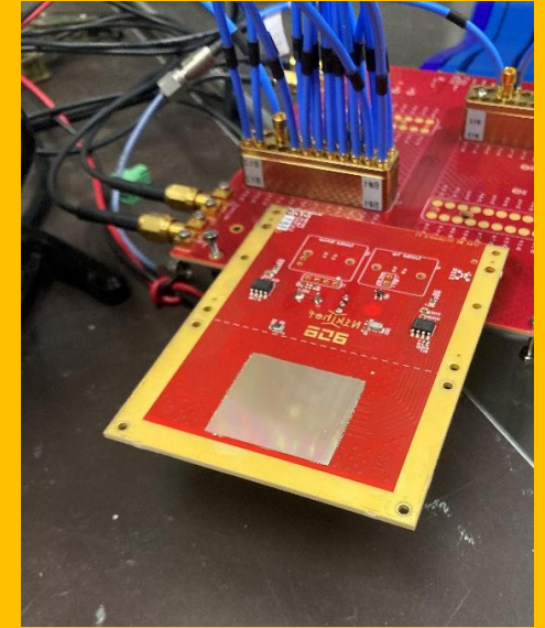
Bonded module connected for electrical testing
