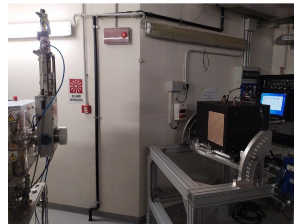
HEPD-02 FM beam test w/ protons @Proton Therapy Trento
