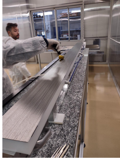
Stiffback-like technique for tube handling, glueing and positioning in the assembly tool
