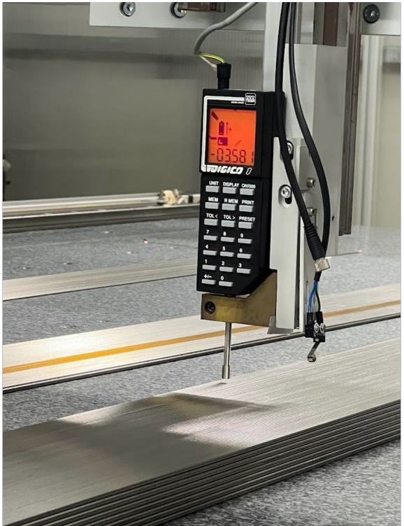
Semi-automatic system for planarity QA/QC
