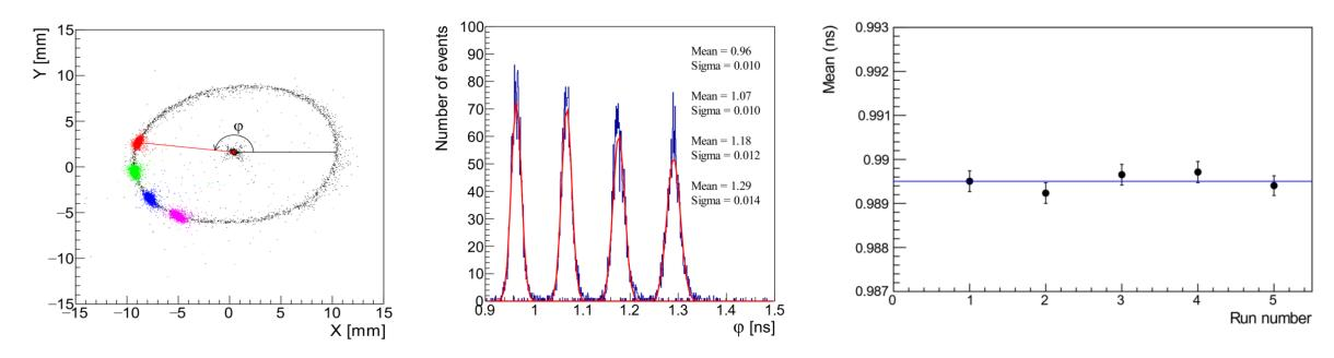
**Left:** 2D image of anode hit positions. The point in the center of the circle is image of electrons with RF turned OFF. The circle is an image of the scanned electrons when the 500 MHz RF is ON, but not synchronized with the laser. The color spots on the circle correspond to phase distributions of the scanned, RF-synchronized photo-electrons for four different fixed phases.
