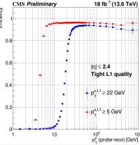
High efficiency also after cleaning of duplicates. High momentum muons go through multiple scattering that reduced the efficiency at high transverse momenta values.
