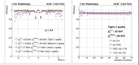
➤ The Muon system illustrates excellent performance across the entire pseudorapidity of the detector and is also stable under the challenging conditions of the Run 3 (>90% efficiency even at high pile-up).
