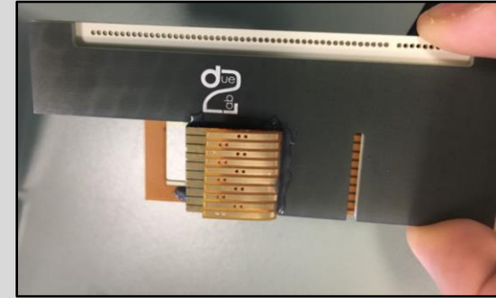
The 3D CZT unit mounted on a support with the I/F for the AFEE
