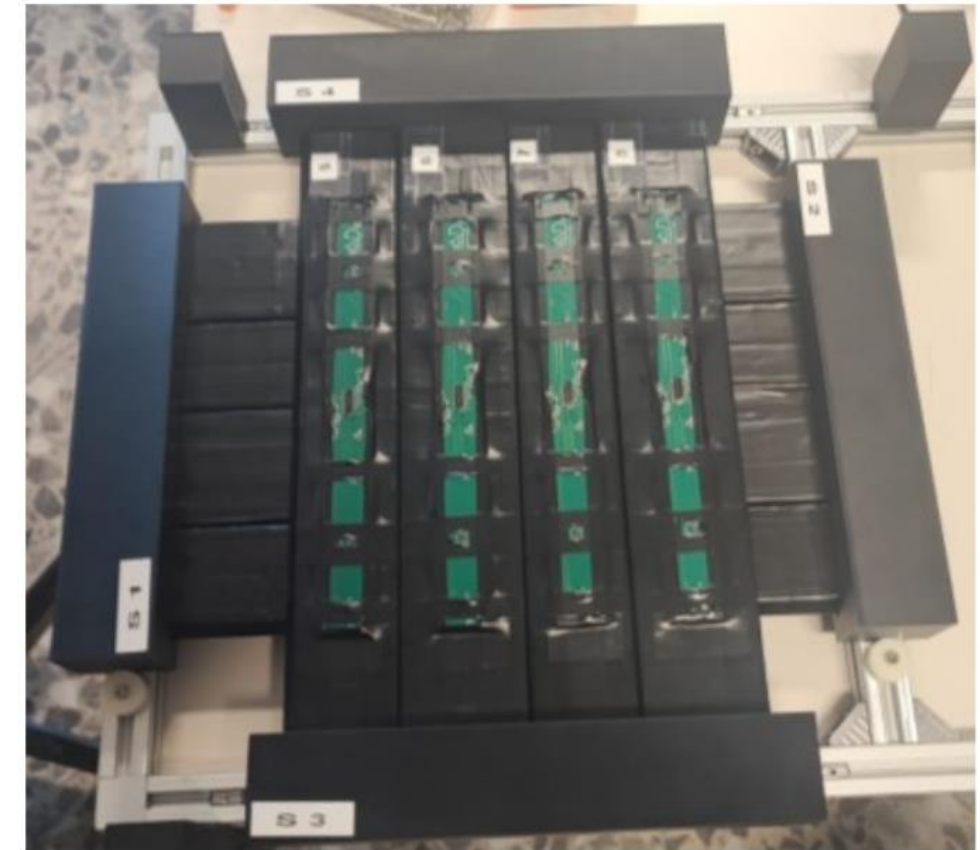
Test beam prototype of the PSD with the PCBs mounted on the bars
