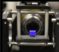
i, CaF 2 crystal, \gamma -irradiated Obj: Mitutoyo 20x/0.28 Color centers induced by \gamma -rays
