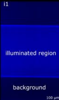
i, CaF 2 crystal, \gamma -irradiated Obj: Mitutoyo 20x/0.28 Color centers induced by \gamma -rays
