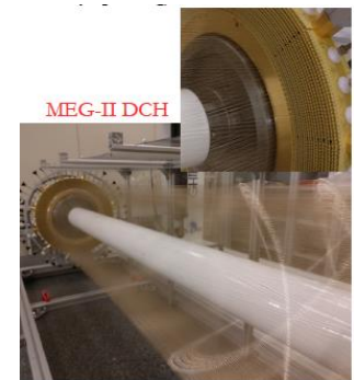
High wire densities prevent the use of feed-through, needing novel approaches to the wiring procedures
