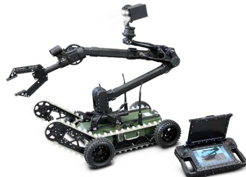
Fig. 1. PIAP GRYF® mobile robot, mobile base on the left, control console on the right.
