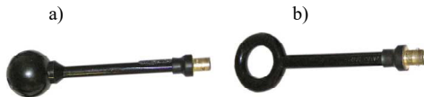
Fig. 12. Near-field probes (ETS-LINDGREN model 7405) used for measurements: a) Type 904 probe, E field, 3 cm ball (omnidirectional), b) Type 902 probe, H field, 3 cm loop.
