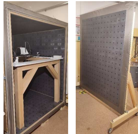
Fig. 8. View of the specialized EMC chamber inside, after filling the walls and doors with ferrite plates. On the left inside the chamber one can see the construction of the EMC scanner.
