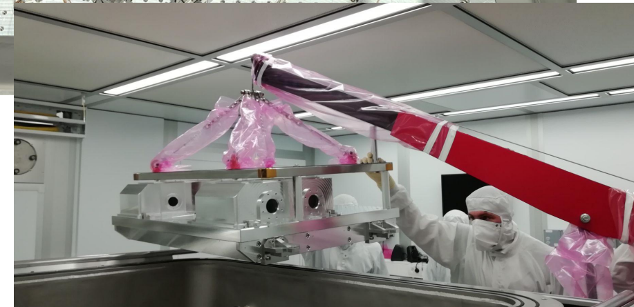
Central Optical Bench in-situ in central vacuum chamber
