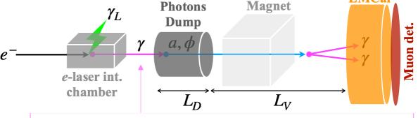
Photons produced in the e-laser collisions are freely propagating to collide with the nuclei of the material of the dump
