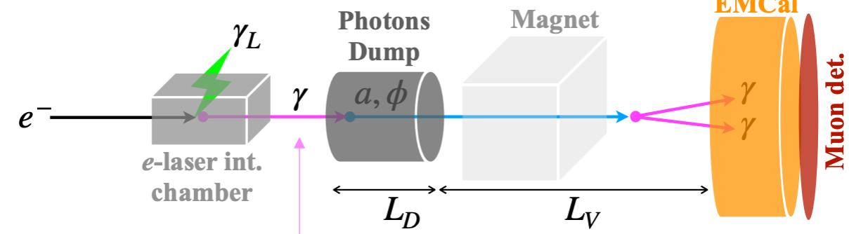
Photons produced in the e-laser collisions are freely propagating to collide with the nuclei of the material of the dump
