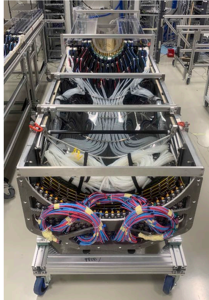
Service routing: several iterations, stripped power cable jackets, added flexible sleeves for power and data cables
