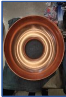
Copper half-Cells production at Jlab for the 5-Cell “clamped” cavity
