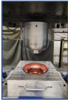
Copper half-Cells production at Jlab for the 5-Cell “clamped” cavity
