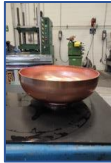
Copper half-Cells production at Jlab for the 5-Cell “clamped” cavity
