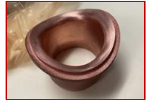
3D-printed HOM port to beam transition- France
