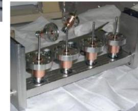
Single-crystal sapphire RF feedthroughs
