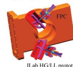
JLab HG/LL prototype cavity HOM endgroup close to FPC
