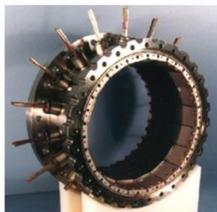
CESR multi-kW cavity beam line absorber
