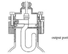
Demountable LEP-type coupler conceived for TESLA cavity
