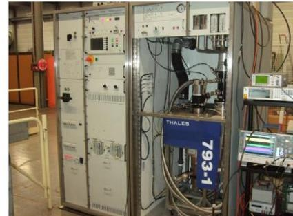
800 MHz IOTs (~60 kW) for the SPS 3<sup>rd</sup> harmonic system
