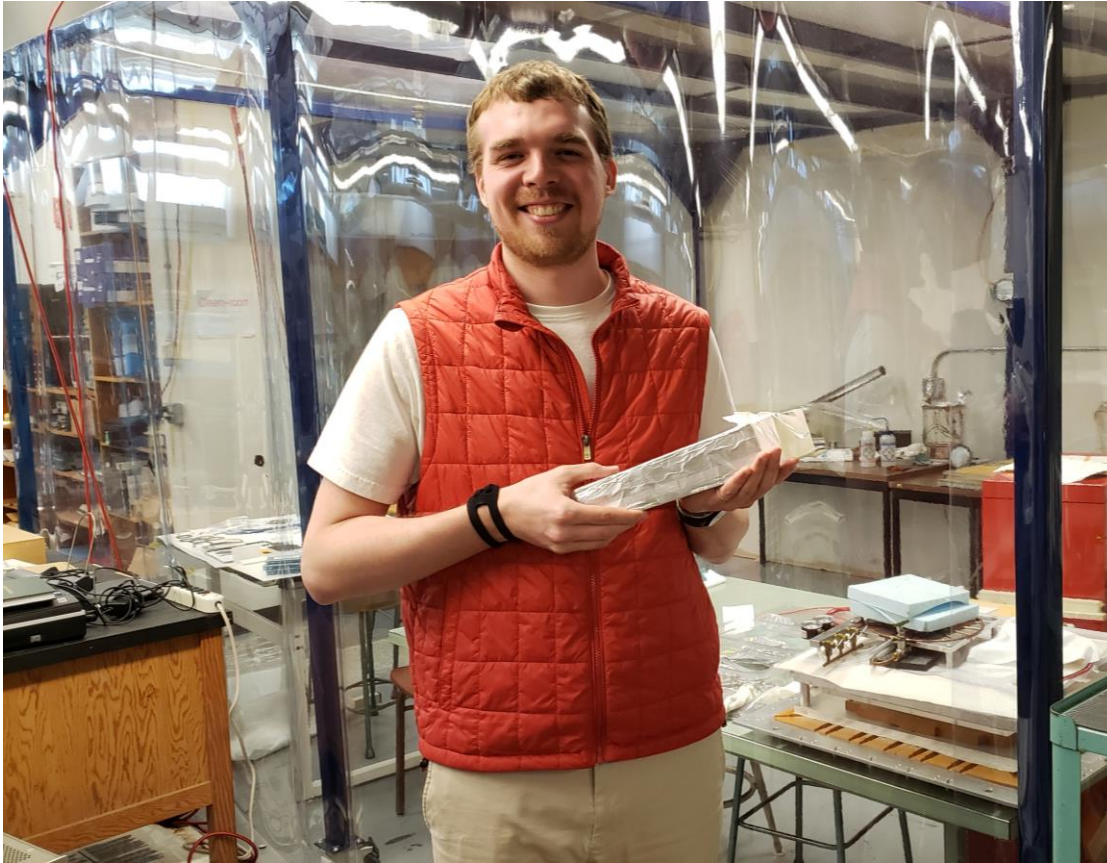
Me holding a spare CsI(Tl) crystal. Belle II's ECL has 8736 of them.
