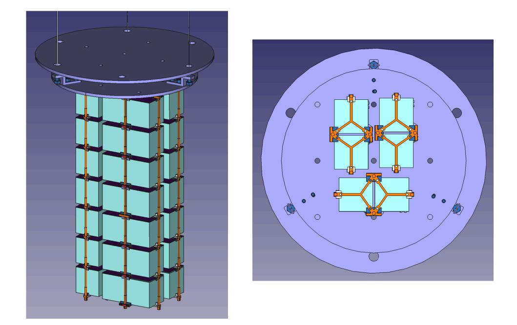
• 42 square Neganov-Luke light detectors with different electrode designs will be used in final demonstrator
