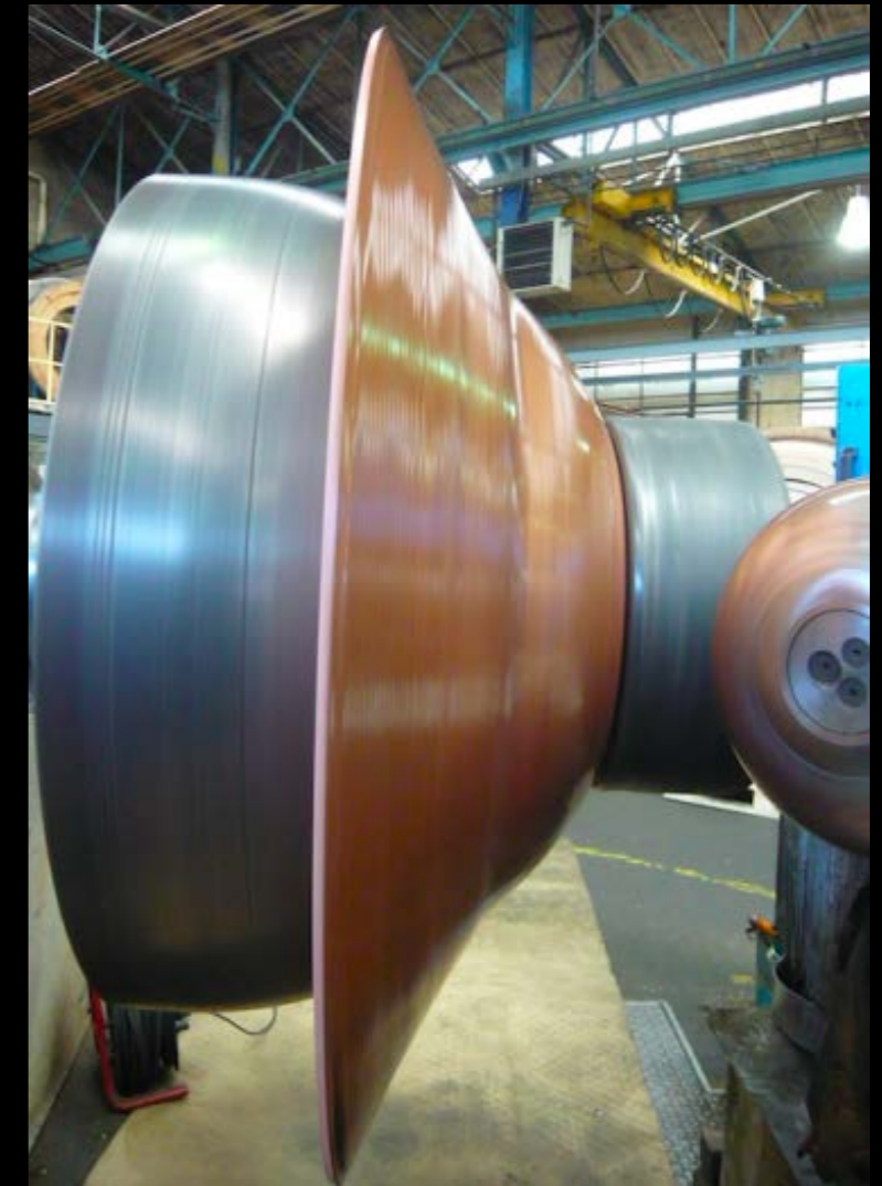
4N Aurubis AG Oxygen Free Copper (99.99% pure) Spun into two hemispheres Electron-beam welded together
