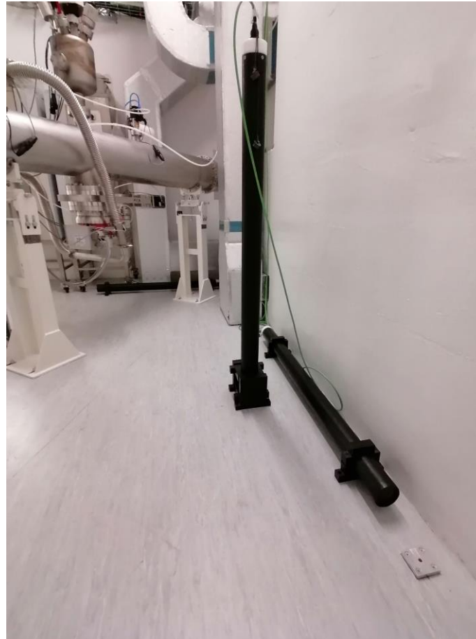
Figure 2. METRONIX Magnetometers (black tubes). One axis each tube.
