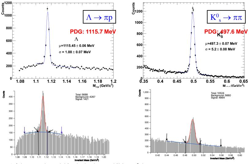
2<sup>nd</sup> degree polynomial for the background  $f(x) = ax^2 + bx + c$ Gaussian for the peak  $f(x) = \frac{1}{\sqrt{2}} e^{-\frac{1}{2} \left(\frac{x-\mu}{\sigma}\right)^2}$
