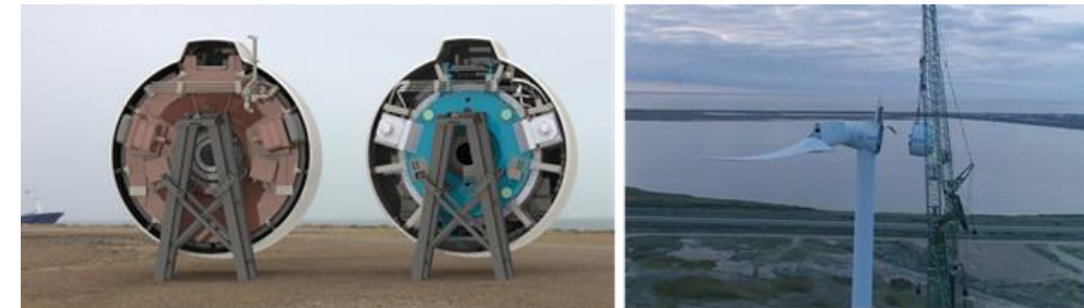
(left) The 3.6 MW EcoSwing HTS generator (blue, 4 m diameter) next to its conventional counterpart with the same power rating (red, 5.4 m diameter), prior to (right) its lift onto the turbine
