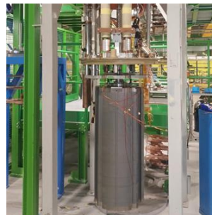
Rotating-coil measurements in SM18
