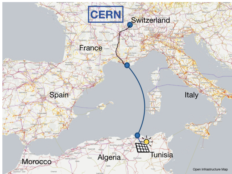
Figure 3.3: Potential CERN-LINK cable (in blue) connecting North African solar power plants with the European electricity grid. Also shown are existing power lines (purple, red, dashed blue), gas and oil pipelines (green/yellow) and PV plants (yellow/red dots). Base map taken from Ref. [69] and annotated.
